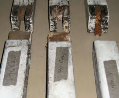
Non-acetylated wood showing severe rot and decay
